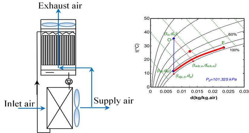
*External IEC coolers with one part of supply air as secondary air*
