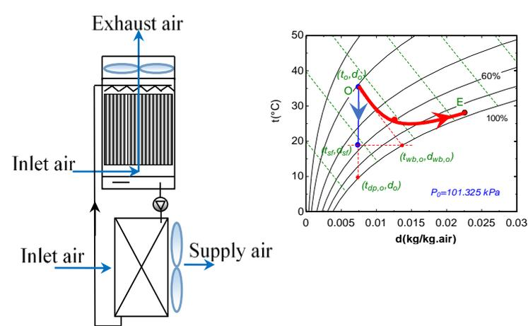
*External IEC coolers with inlet air as secondary air*
